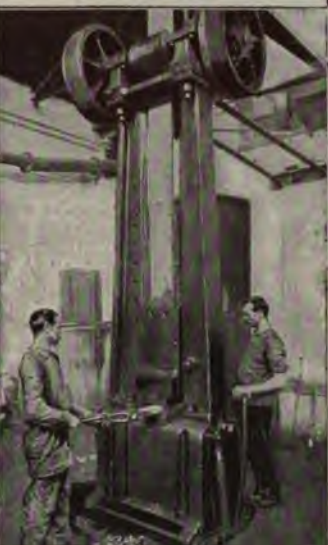
2. Making gun barrels. A solid bar of metal is heated and hammered until it is tempered and in shape. It is afterward bored out. This is a steam trip hammer used to forge the metal.
